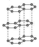
It has  $sp^2$  hybridised carbon, arranged in the form of layers. These layers are held together by weak van der Walls' forces. These layers can slide over each other, making graphite soft and slippery. Therefore, it is used as a lubricant.
