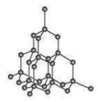
The rigid 3-D structure of diamond makes it a very hard substance. In fact, diamond is one of the hardest naturally-occurring substances. It is used as an abrasive and for cutting tools.
